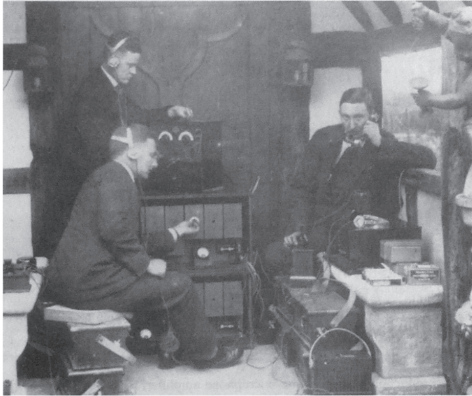
Figure 8.3 Two Marconi GA1 microphone amplifiers installed for a 1925 outside broadcast of the song of the nightingale from a Surrey wood. A 6 V battery and six wooden boxes containing 50 V batteries may be seen.
